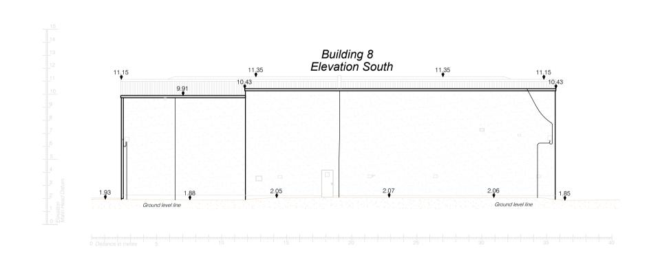
Demolition Works - Elevations (Building 8) scale 1:200 @ A1
